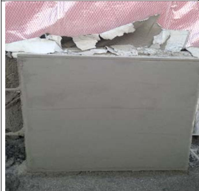
1 of 3 panels cast for shotcrete testing
