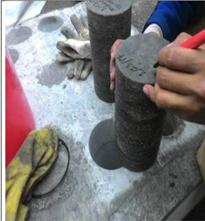
Coring and marking concrete samples from shotcrete panels
